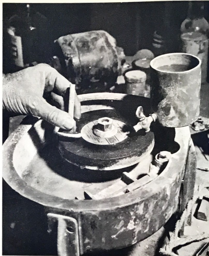
Here Mac Myers polishes a Georgia jewel on the wheel of a lapidary machine. The stone is fastened to a "dop stick" with sealing wax.
